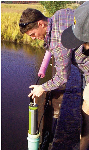
Dissolved oxygen is measured with oxygen sensors.
